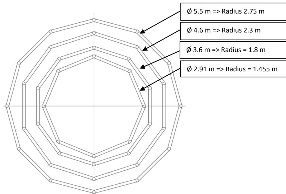
**The slab dimensions must exceed the pool dimensions by at least 30 cm all around the pool.**
